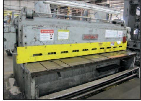
CINCINNATI # 2510 POWER SHEAR 10' X 3/8" CAPACITY
