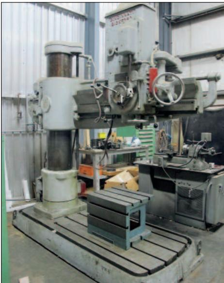
CINCINNATI-BICKFORD # 4E RADIAL DRILL, 6'X 15" CAPACITY
