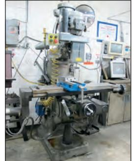
BRIDGEPORT 1.5 HP VERTICAL MILL W/ EZ-TRAX DX CNC CONTROL
