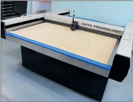
DATA TECHNOLOGY CNC SAMPLE CUTTING TABLE MODEL DPS6648
