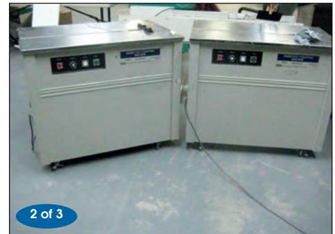
Uline Poly Strapping Machine Portable Model H-959
