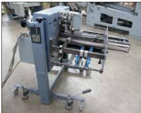
Stahl Air Knife Fold Unit Model VFZ52
