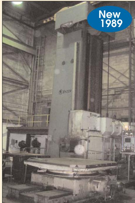
SKODA #W-200HC 7.87" CNC FLOOR TYPE HORIZONTAL BORING MILL
