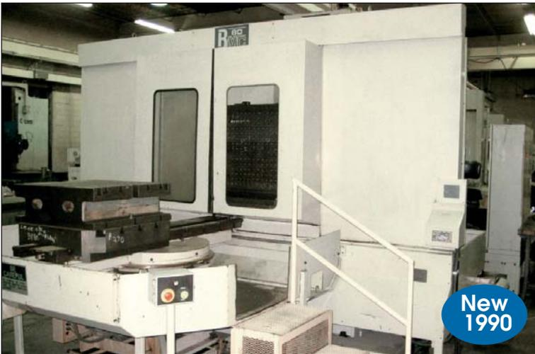
TOSHIBA SHIBAURO #BMC-80 CNC HORIZONTAL MACHINING CENTER
