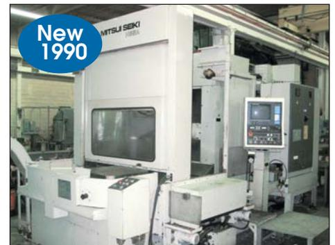
MITSUI-SEIKI MODEL HS-5A "5-AXIS" HORIZONTAL MACHINING CENTER, FANUC 15M, #CT-50 TAPER
