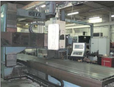
OOYA #5M BRIDGE TYPE VERTICAL MACHINING CENTER #CT-50 TAPER
