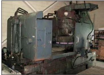
1968 BLANCHARD MDL #32-60 ROTARY SURFACE GRINDER, 60" MAGNETIC CHUCK
