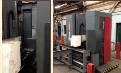
Voortman #V-600 CNC Beam Drilling System with View of Feed Table & Interior
