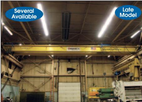
Dwight Foote 5 Ton Bridge Crane, w/ Dual 5 Ton Hoists
