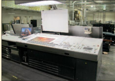
Heidelberg 6 Color Sheet Fed Printing Press Model CD102-6+L, S/N 540399, Extended Delivery, Vario Dampening, Closed Loop with Intellitrac Scanner, Grafix Powder Coat Delivery, Auto Plate Changers, Auto Blanket Washers, Roll Coater, 161 Million Impressions, CPC 104 Console, IR Dryer and Air Knives, Plate Punch
