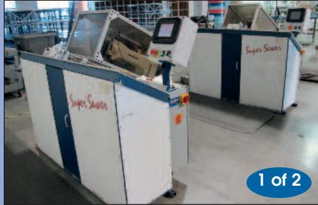
ODM Sewer Model Super Sewer, S/N SN-1107, w/ Seiko Sewing Machine Head
