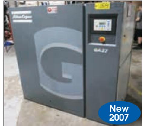
ATLAS COPCO 50 HP ROTARY SCREW COMPRESSOR MODEL GA37
