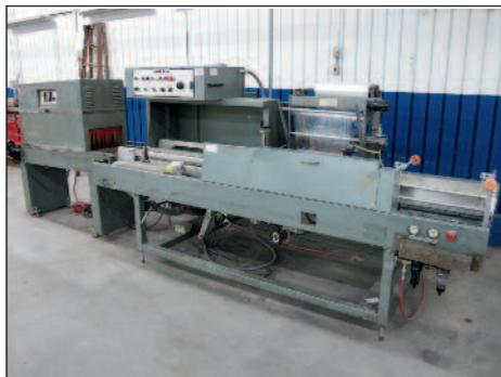
Weldotron L-Seal Packaging Machine Model 9511F
