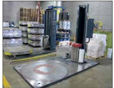
LANTECH & WULFTEC ROTARY STRETCH PALLET WRAPPERS
