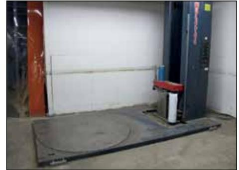
WULFTEC ROTARY STRETCH PALLET WRAPPER
