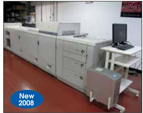
CANON DIGITAL PRINT PRODUCTION SYSTEM MODEL IMAGEPRESS C7010VP
