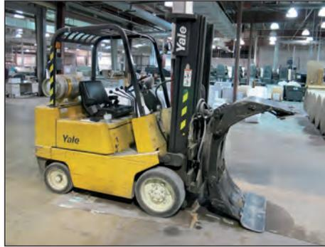
YALE 5000 LB LPG FORKLIFT, TRIPLE MAST W/ROLL CLAMP
