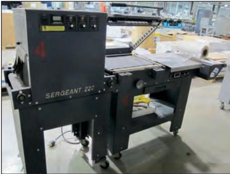
SERGEANT L-SEAL PACKAGING MACHINE MODEL 220 W/HEAT TUNNEL
