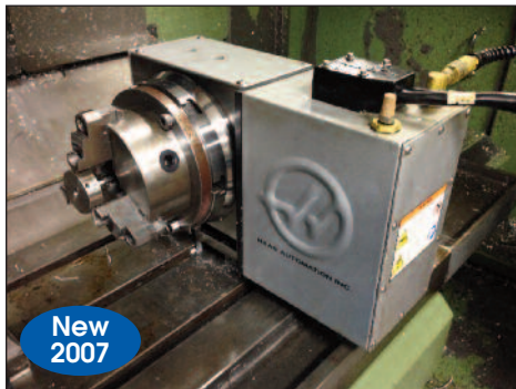
HAAS CNC 4th-Axis Rotary Table w/ Brushless HAAS Control
