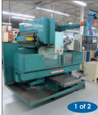
Matsuura #MC-760V CNC Vertical Machining Center
