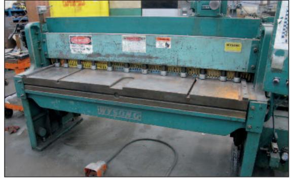
WYSONG SHEAR MODEL 1272, 12 GAUGE CAPACITY, 6'
