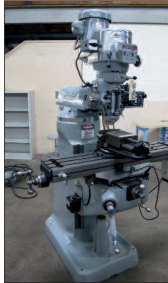
BRIDGEPORT 2 HP SERIES 1 VERTICAL MILL, S/N 141958, POWER FEED, SWI DRO
