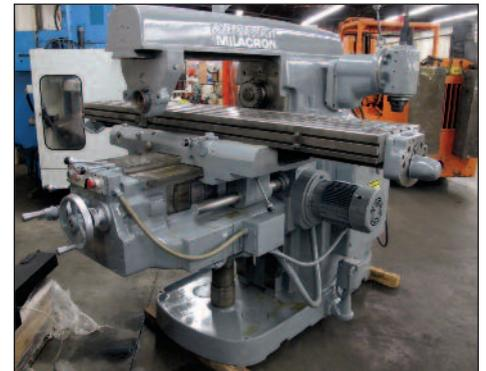
CINCINNATI HORIZONTAL UNIVERSAL MILLING MACHINE MODEL 415-16, DIAL TYPE
