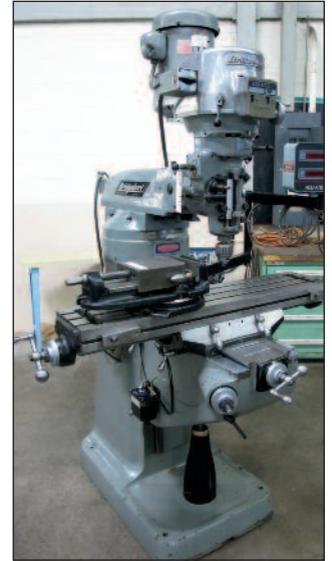
BRIDGEPORT 2 HP SERIES 1 VERTICAL MILL, S/N 243643, POWER FEED, ACCURITE DRO
