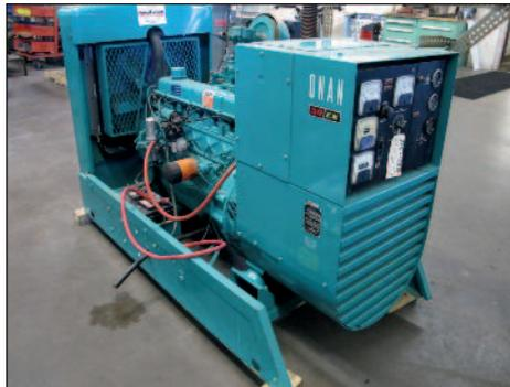
ONAN ELECTRIC GENERATOR SET # 30EX-30.0EK-15R/1786H, 3 PHASE, 35 KW, 1 PHASE, 20 KW, 725 HOURS
