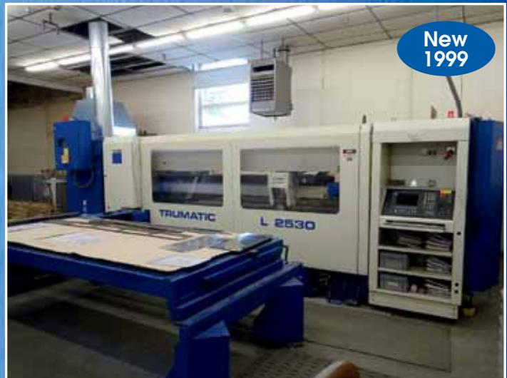
Trumpf Trumatic Laser Cutting System Model L2530
