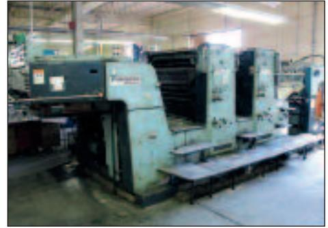
Planeta 2/C Sheet Fed Printing Press Model Super Variant P24 SW
