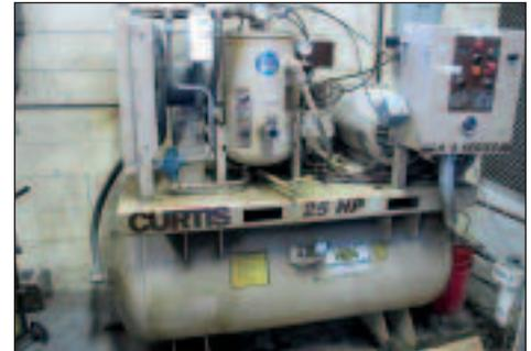
Curtis 25 HP Rotary Screw Compressor Model RS25A
