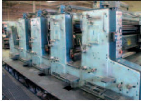
Planeta 4/C Sheet Fed Printing Press Model Super Variant P45 SW2
