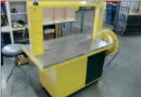
Strapack Automatic Strapping Machine Model RQ-8
