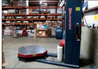
Wulftec Rotary Stretch Pallet Wrapper Model WHP-200
