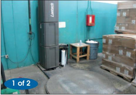
LANEtech ROTARY STRETCH PALLET WRAPPER MODEL Q SERIES
