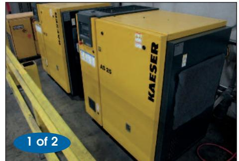
KAESER ROTARY SCREW AIR COMPRESSOR MODEL AS25
