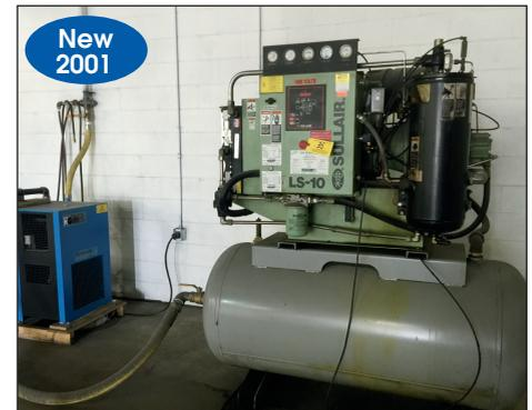
SULLAIR 40 HP ROTARY SCREW AIR
