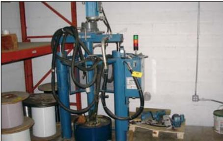
NORDSON BULK MELTER APPLICATOR MODEL 5506
