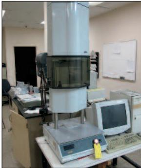
Kayness Capillary Rheometer Model D6052M-115
