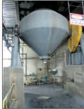
175 CuFt Patterson Kelly, Jacketed Conical Rotary Vacuum Dryer
