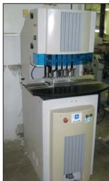
Baum 5-Spindle Drill Model D5-A-3
