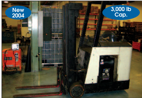
Crown # RC-3020-30 Stand Up Riding Type Electric Forklift
