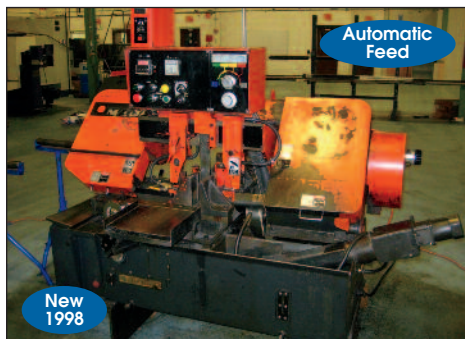
Amada #HA-250W Automatic Horizontal Band Saw
