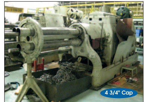
Acme Gridley # RA-4 (4-Spindle) Automatic Multi-Spindle Screw Machine
