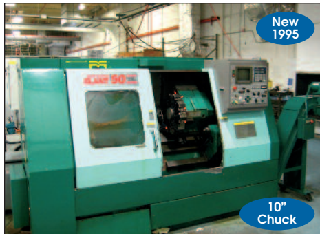
Methods Slant 50 CNC Slant Bed Turning Center
