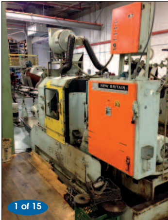
New Britain-Gridley # 51 (6-Spindle) Automatic Multi-Spindle Screw Machine
