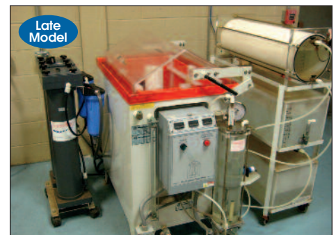
Singleton # SCCH-20 Salt Bath Corrosion Test Chamber
