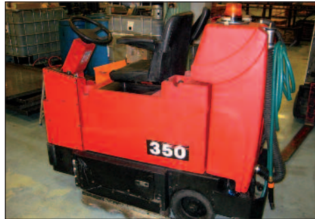
R.P.S. # 350 Electric Riding Type Floor Scrubber
