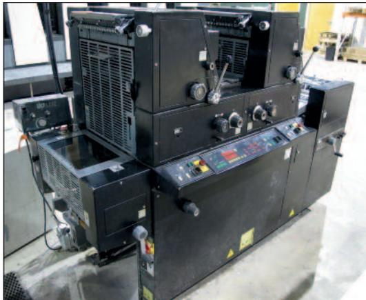
AB Dick 2/C Offset Press #9985, S/N L8492, Crestline Dampening, Airtech Ultra Air Powder System
