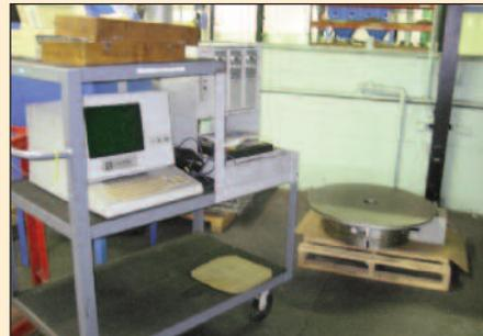
PNEUMO AIR BEARING ROTARY GAGE W/ Controls
