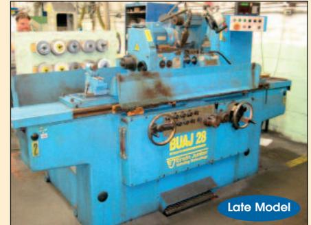
ERWIN JUNKER # BUA-J28 14" x 40" Cap. "Universal" Cylindrical Grinder W/ Swivel Workhead, 3-jaw chuck, Wheel Balancer, Sony DRO, Steadyrest, Universal Swivel Table, S/N 357107
