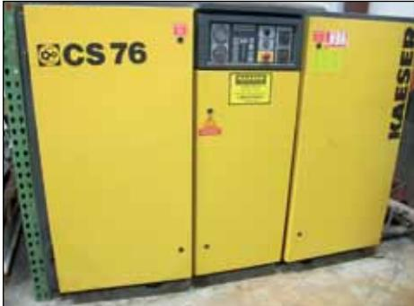
KAESER 60 HP ROTARY SCREW AIR COMPRESSOR MODEL CS76
