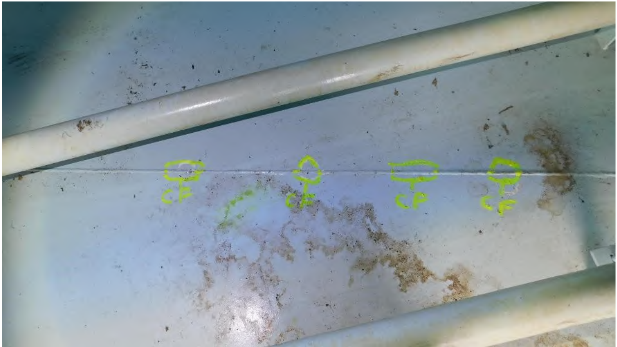
Photograph 25: Bottom Plate Weld Coating Failure Overview
