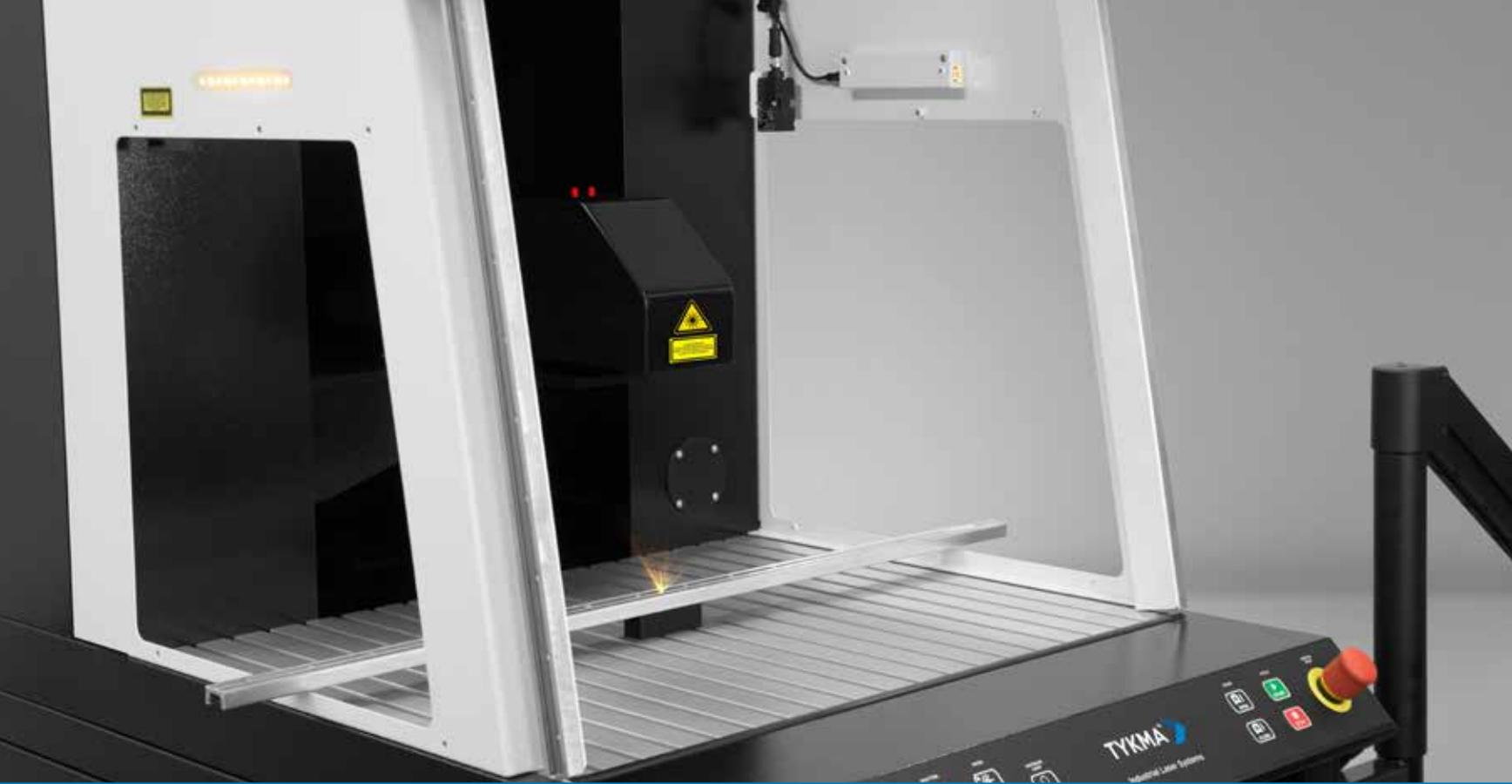
Zetalase™ XL offers an expansive work area and is highly configurable for a variety of applications. Zetalase™ XL is ideal for the processing of tall and/or large components as well as large fixtures of parts. A front vertical patented pneumatic safety door maximizes operator ergonomics. A choice of laser power and a variety of accessories and customizations provide the ability to solve any application.
