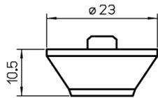
Dyshållare/nozzle holder passande Precitec, Precitec KT M1.5" S F2.5
