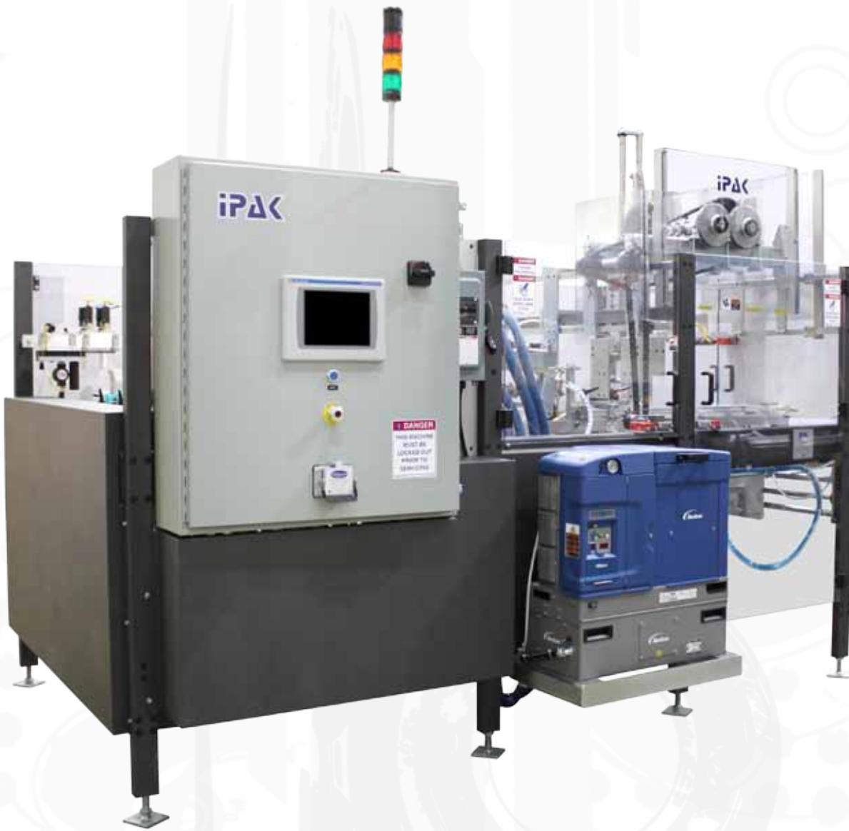
IPak's Model TF-200Q fully automatic tray former is designed and built to withstand the rigors of continuous, heavy-duty, industrial applications. The TF-200Q will form regular slotted trays in various configurations including four corner glued trays, one and two piece telescoping trays, and variations of self-locking trays suitable for most any application including agricultural, food processing and distribution. It will continuously operate at speeds of up to 35 trays per minute and is capable
