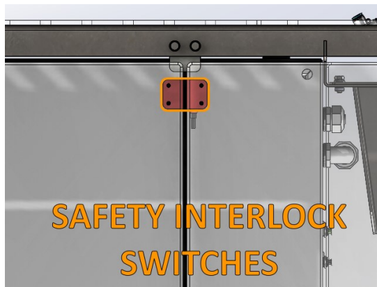
Figure 4 - Safety Interlock Doors
