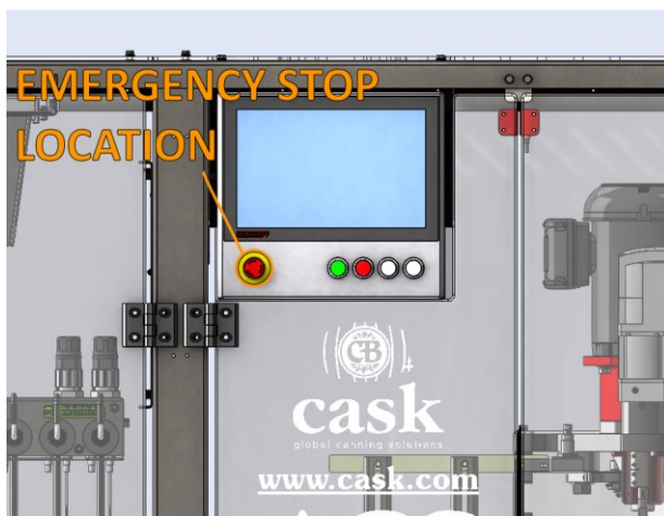
Figure 5 – Emergency Stop Location
