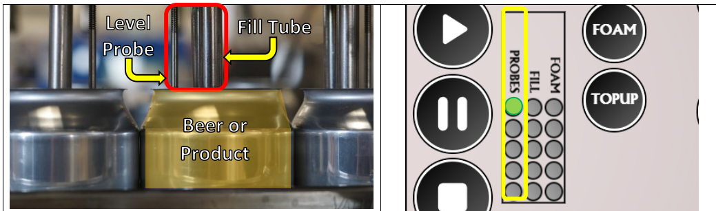
When Product fills the cans and both the fill level probes and the fill tubes are both touching the liquid, the signal will be sent to the PLC to stop filling. You can see when this signal is made by observing green lights illuminating the "Probes" section on the "Run" page.
