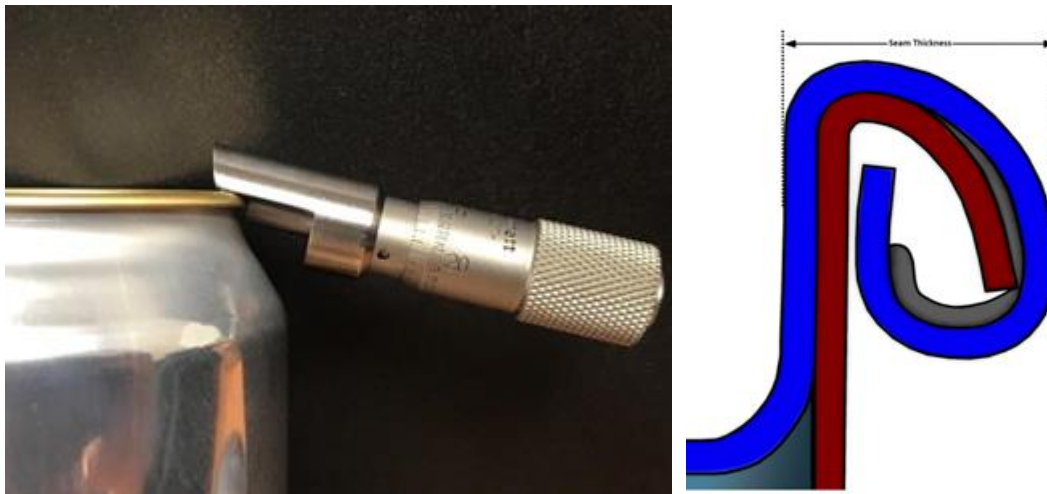
Figure 21 Micrometer positioned on can for measuring 1st Op Thickness
