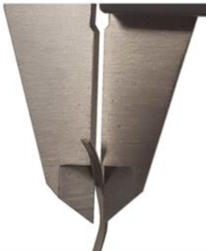
Figure 37 Measuring the Cover Hook using digital Calipers
