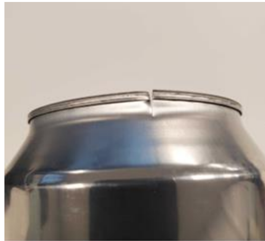
Figure 35 Notch cut in can seam for cover hook removal
