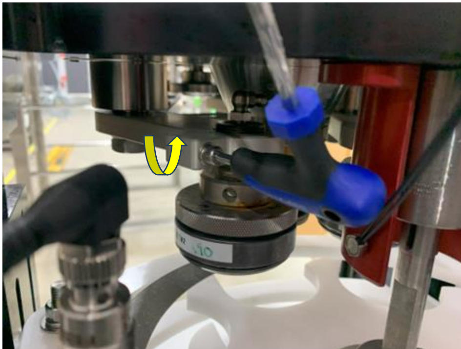
Figure 13 Loosening the Vertical Adjustment Socket
