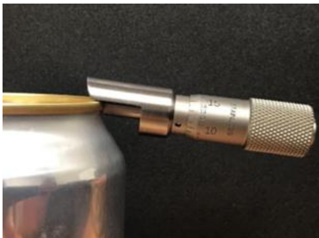
Figure 31 Micrometer positioned on can for measuring 2 nd Op Thickness
