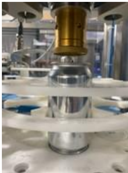
Figure 10 Empty Lidded Can on Lift Table
