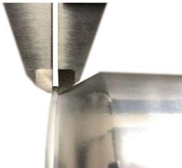
Figure 39 Measuring the Cover Hook using digital Calipers
