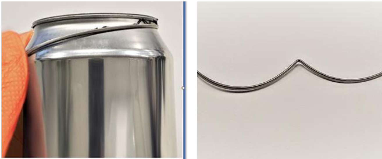
Figure 36 Pulling the Cover Hook down & Cover Hook removed
