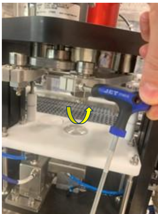
Figure 17 Counterclockwise turn on seaming arm (5/32 Allen Wrench or 5mm Metric)
