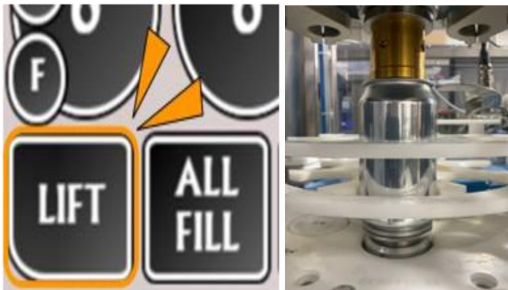
Figure 11 Lift Button (HMI) & Lifted Can on Seamer
