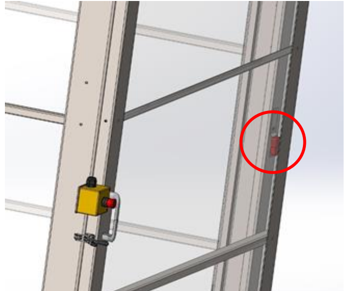
Figure 3 - Interlock Mechanism (Highlighted) - Door Closed
