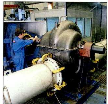
Performance and Pulsation Test Station.
