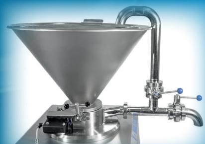
The PVS-Micro-Cut cutting system, based on the rotor/stator principle, operates absolutely contact free without any metal abrasion. The cutting tools made of high quality chromium nickel steel are equipped with special cutting inserts ensuring a high throughput capacity.
