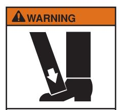
Rotating head can fall when removing or installing. Serious injury can result.
