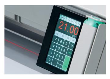
TOUCH PAD Extremely convenient and easy-to-use: Electronic control module for the power back gauge with multilingual touch pad. 99 programs with up to 99 steps can be stored. Also useful: the pre-programmed DIN sizes and the automatic memory for repeat cuts.
