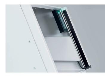
IR LIGHT BEAM SAFETY CURTAIN Efficient and safe cutting and trimming is guaranteed by the IR light beam safety curtain on the front table. Additional safety is provided by the transparent safety cover on the rear table.
