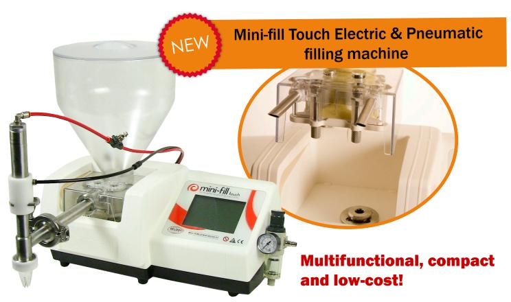
Compact ELECTRIC / PNEUMATIC filling/injecting machine with a TOUCH SCREEN incl. safety glass This filling machine is designed for SPOT, STRIPE depositing, INJECTING and DECORATION
