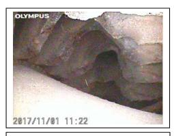
Rotor tapers are completely eroded.
