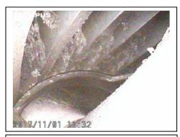
Idle end: Rotor is in near new condition.
