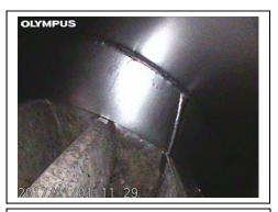
Idle end: Head shroud, body liner and rotor viewed here at the head. All good..!!!!
