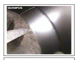
Drive end: Seen here towards the center shroud, tight measurement and smooth surfaces.
