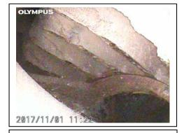
From another angle, eroded tapers, cone edge at the discharge is also worn.
