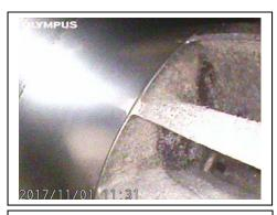
Idle end: close-up view of the center shroud to rotor clearance; very tight measurement.
