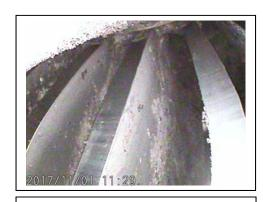
Drive end: Viewed here are three rotor blade tapers; all are square, even and true. Rotor is Stainless Steel cast.
