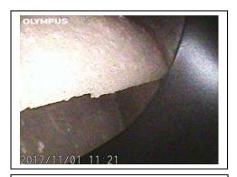
Rotor blade OD is eroded. Head shroud is acceptable.
