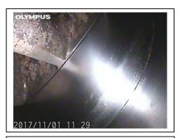
Drive end: below in the compression area, all surfaces are smooth and clean. Head shroud to rotor clearance is tight.
