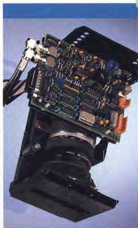
High speed CCD camera captures visual web defects faster than the human eye.
