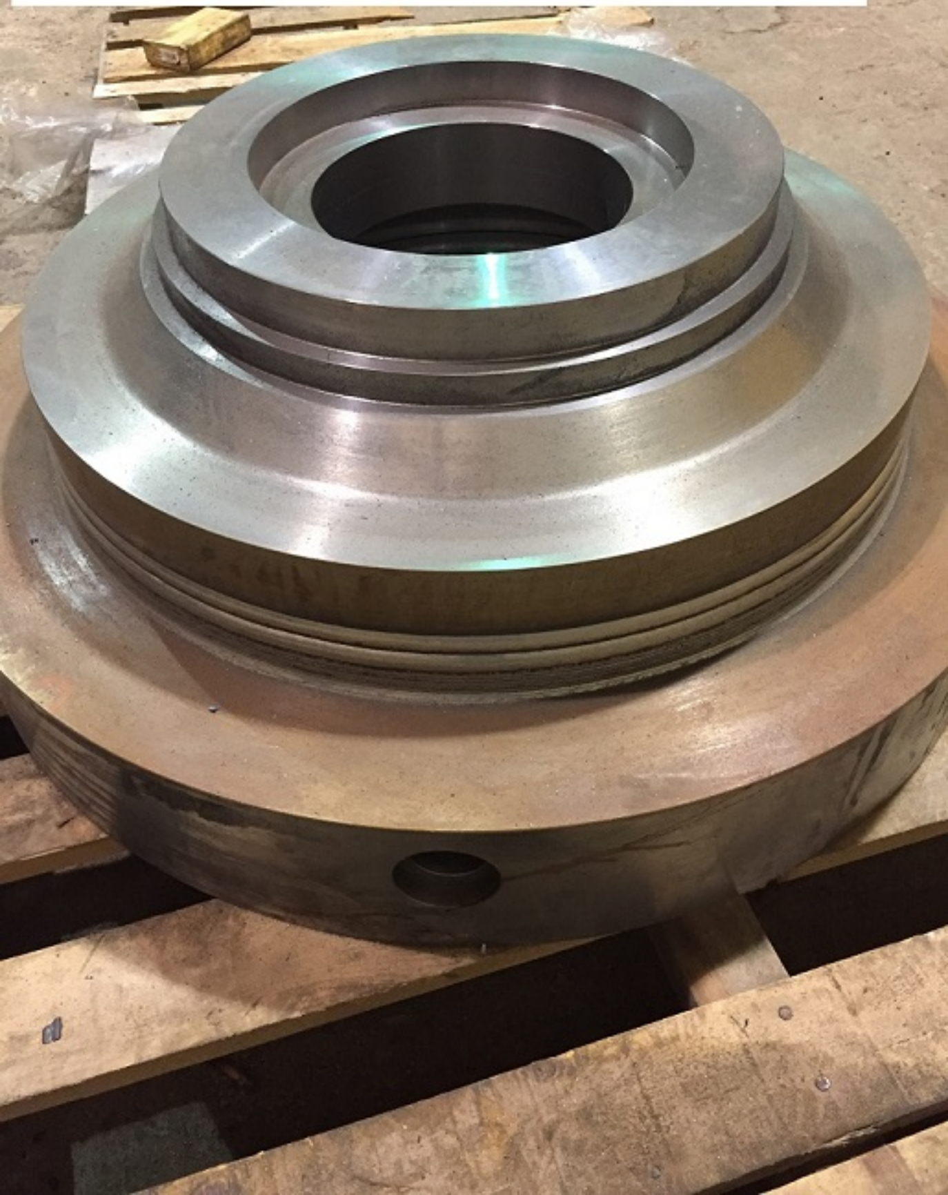
DISCHARGE HEAD AFTER WELDING DIFFUSER SPACER
