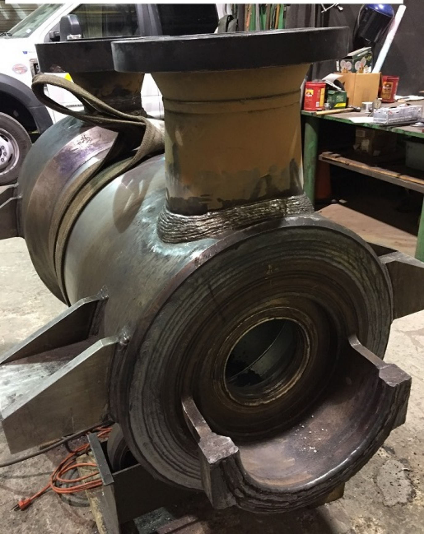
BARREL AS WELDED PRIOR TO STRESS RELIEVE
