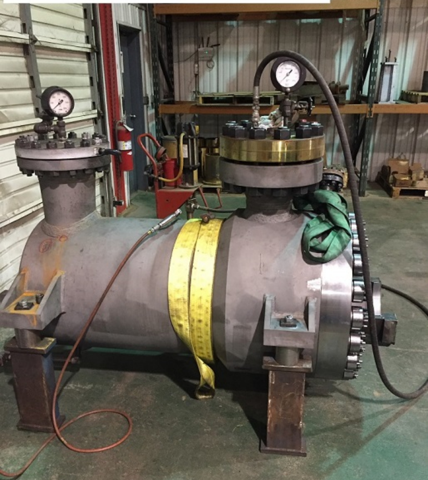
BARREL HYDRO, 3300 PSI HP, 675 PSI LP
