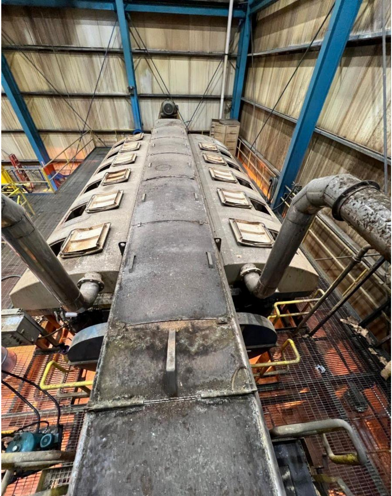
Metso Twin Roll Press, Model TRPW-1572, S/N P-09503, Mfg. 2005, 1.5md X 7.2ml Rolls, Hydraulic Drive w/ 400 HP Toshiba Motor, Auxiliary Hydraulic Power Unit and Vertical Hydraulic Pump Set
