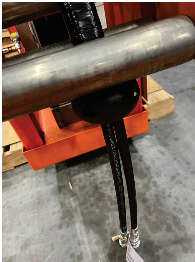
Figure 4-30: Removing the Hose Bumper on the Hydraulic Hose
