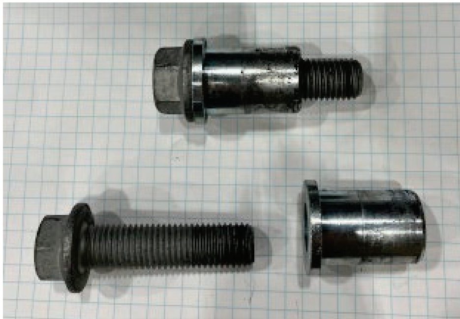
Figure 4-4: Transport Anchor Bolts – Bolt and Sleeve
