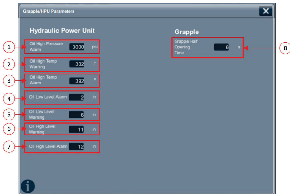
Figure 5-49: Grapple Hoist – HMI Grapple Shovel and HPU Parameters Screen
