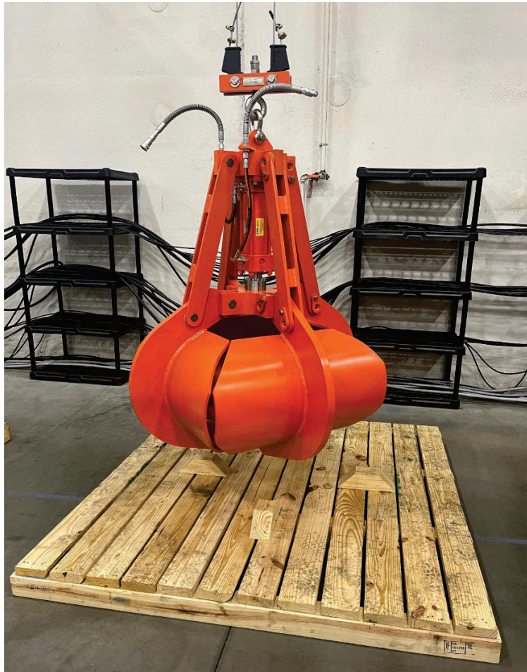
Figure 4-24: Applying Load to the Wire Rope Fastening Point
