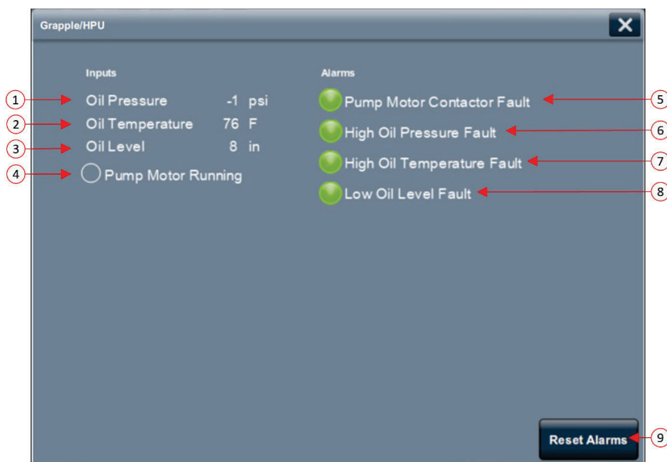
Figure 5-39: Grapple Hoist - HMI Grapple Shovel and HPU Sensors Screen
