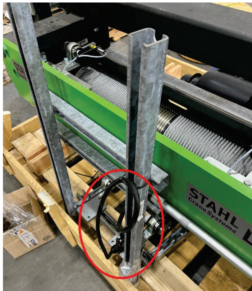
Figure 4-5: Paddle Limit Switch Assembly – Location
