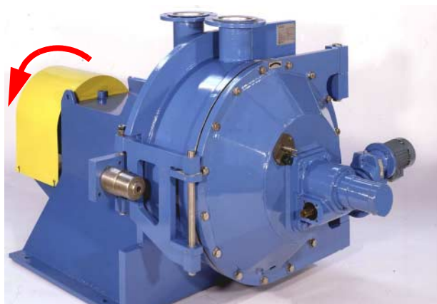
Fig. 5-9 Sense of rotation of the machine
