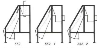
STANDARD 552 Standard headbox, flanged effluent discharge 552—1 Deep headbox, wide effluent discharge 552—2 Deep headbox, flanged effluent discharge
