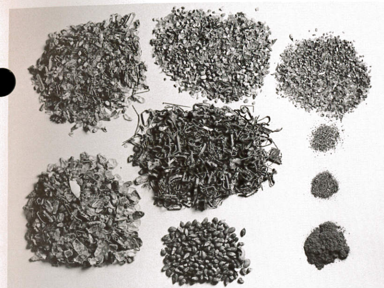
Debris removed with a Liquid Cyclone from 4% stock; DP = 20 PSI (138 kPa).
