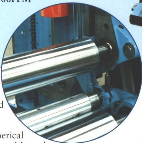
Cameron Type 420 Width 92" Rewind Diameter 50" Speed 2500FPM
