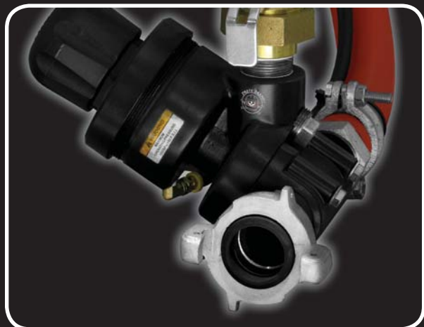
Full port blast hose couplings reduce restriction at crucial connection points for increased air/abrasive flow.
