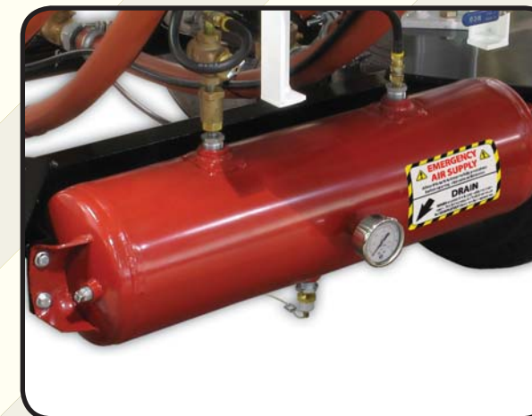
The Emergency Air Supply tank is used on SPH PINCH systems to ensure that the Pinch Valves can not open in the event of an air source failure.
