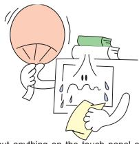
Never put anything on the touch panel or around it. Otherwise, ventilation will be restricted, causing the temperature in the machine to rise, resulting in failure.
